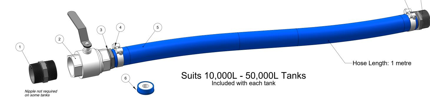
Note: Flex Connection Kit (Included with each tank) must be used on the outlet to maintain warranty. Refer Tank Installation Guidelines.
