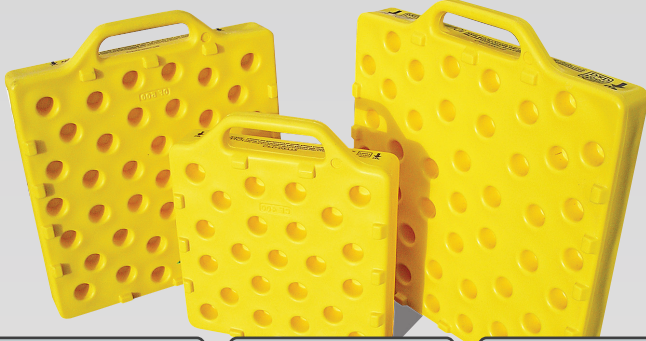
Cranefoot 500 Length: 560mm Width: 500mm Height: 85mm Rated at 10 tonne FMAM400.1010
