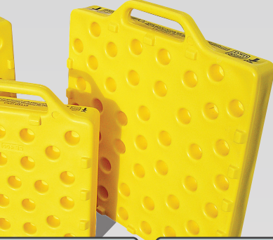
Cranefoot 400 Length: 450mm Width: 390mm Height: 85mm Rated at 6 tonne FMAM400.1020
