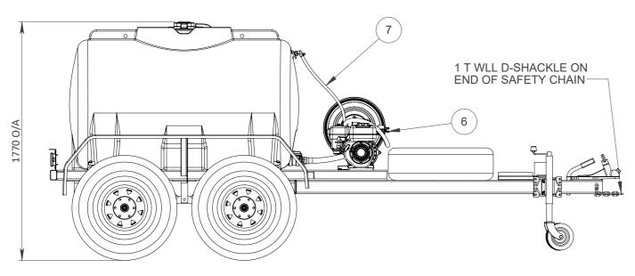
TARE WEIGHT - (625 EST) kg APPROX ATM (AGGREGATE TRAILER MASS) - (2,125 EST) kg APPROX TOW BALL WEIGHT (FULLY LOADED) - (195-205 EST) kg APPROX
